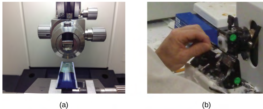
Figure 2.42 (a) An ultramicrotome used to prepare specimens for a TEM. (b) A technician uses an ultramicrotome to slice a specimen into thin sections. (credit a: modification of work by “Frost Museum”/Flickr; credit b: modification of work by “U.S. Fish and Wildlife Service Northeast Region”/Flickr)
