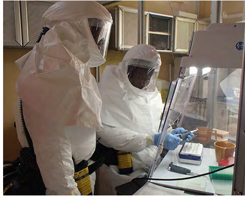
Figure 6.15 Researchers working with Ebola virus use layers of defenses against accidental infection, including protective clothing, breathing systems, and negative air-pressure cabinets for bench work. (credit: Randal J. Schoepp)
